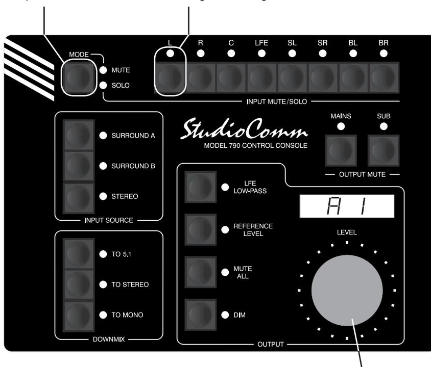
Use the Level control to change this specific Model 790's device address. Address can be either A1, A2, A3, or A4. See Note below.
