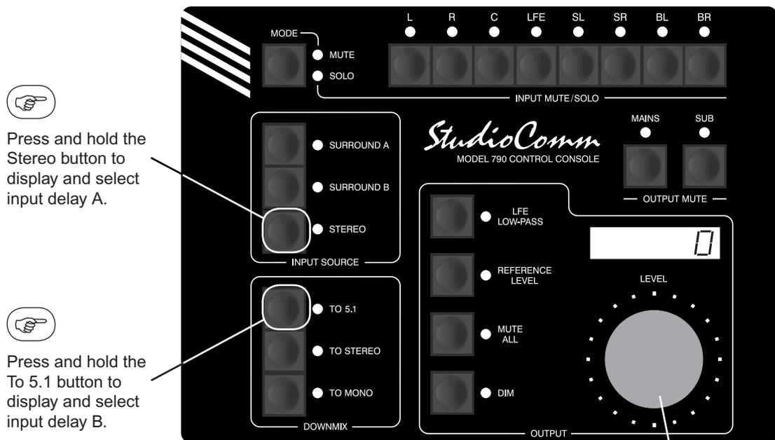
Use the level control to adjust the input delay. Range is from 0 to 340. The display shows delay in milliseconds at 48 kHz sampling rate. The value is scaled up or down for other sample rates.
