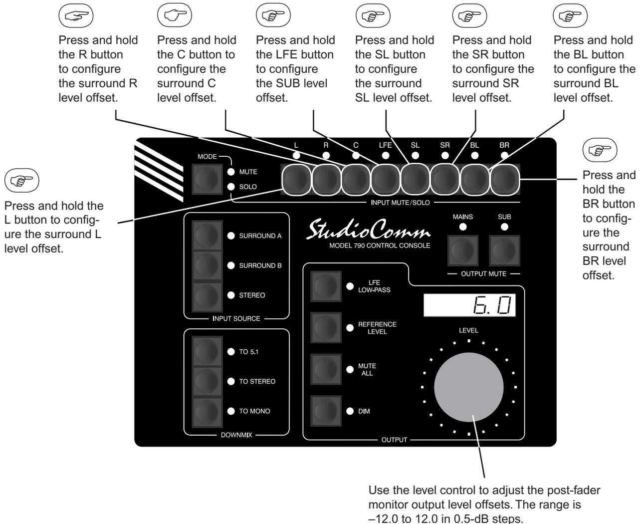
**Default:** 0.0 dB post-fader monitor output level offsets.
